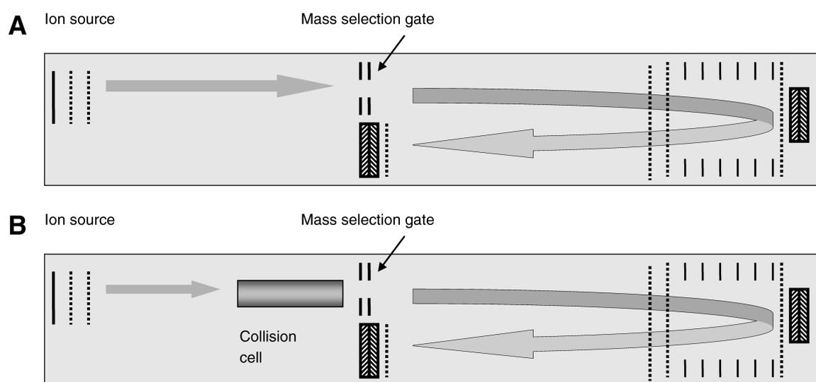
Fig. 1. Schematic of the AXIMA CFR mass spectrometer using (A) laser-induced dissociation or (B) collision-induced dissociation.
