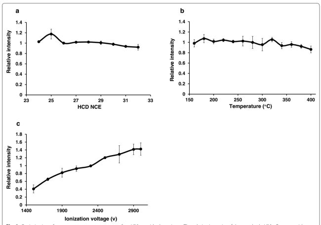
Fig. 2 Optimization of mass spectrometry parameters for pY39 peptide detection. **a** The relative intensity of the standard pY39 αβ-syn peptide with different HCD NCEs. **b** The relative intensity of the standard pY39 αβ-syn peptide with different ion transfer tube capillary temperatures. **c** The relative intensity of the standard pY39 αβ-syn peptide with different ESI voltages
