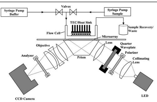
Fig. 1 Schematic drawing of the LFIRE™ optical setup and associated liquid handling for the flow cell configuration
