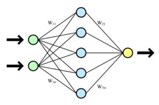
Fig. 3. A schematic representation of an artificial neural network.
