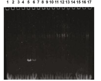
**Figure 2** Mini gel SDS-PAGE analysis of protein fractions resulting from PIEF using a known protein, beta lactoglobulin, and a pH 3-10 IPG strip (gel stained with Sypro Ruby). Lanes 1-17: fractions from paper strips 1-17.
