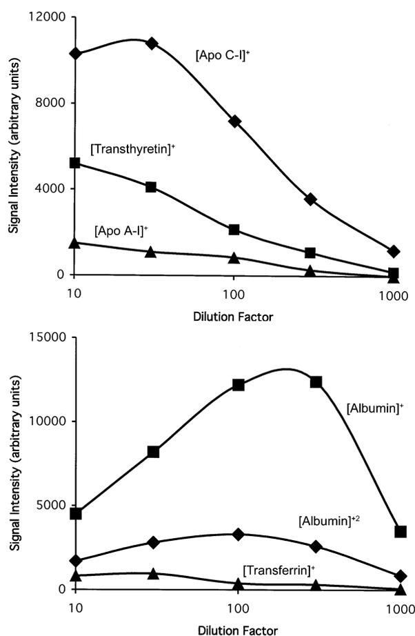
Fig. 4. Peak intensities (peak heights) with varying dilution of serum. Listed dilutions reflect dilution with 10 mM ammonium acetate prior to further threefold dilution with matrix solution.
