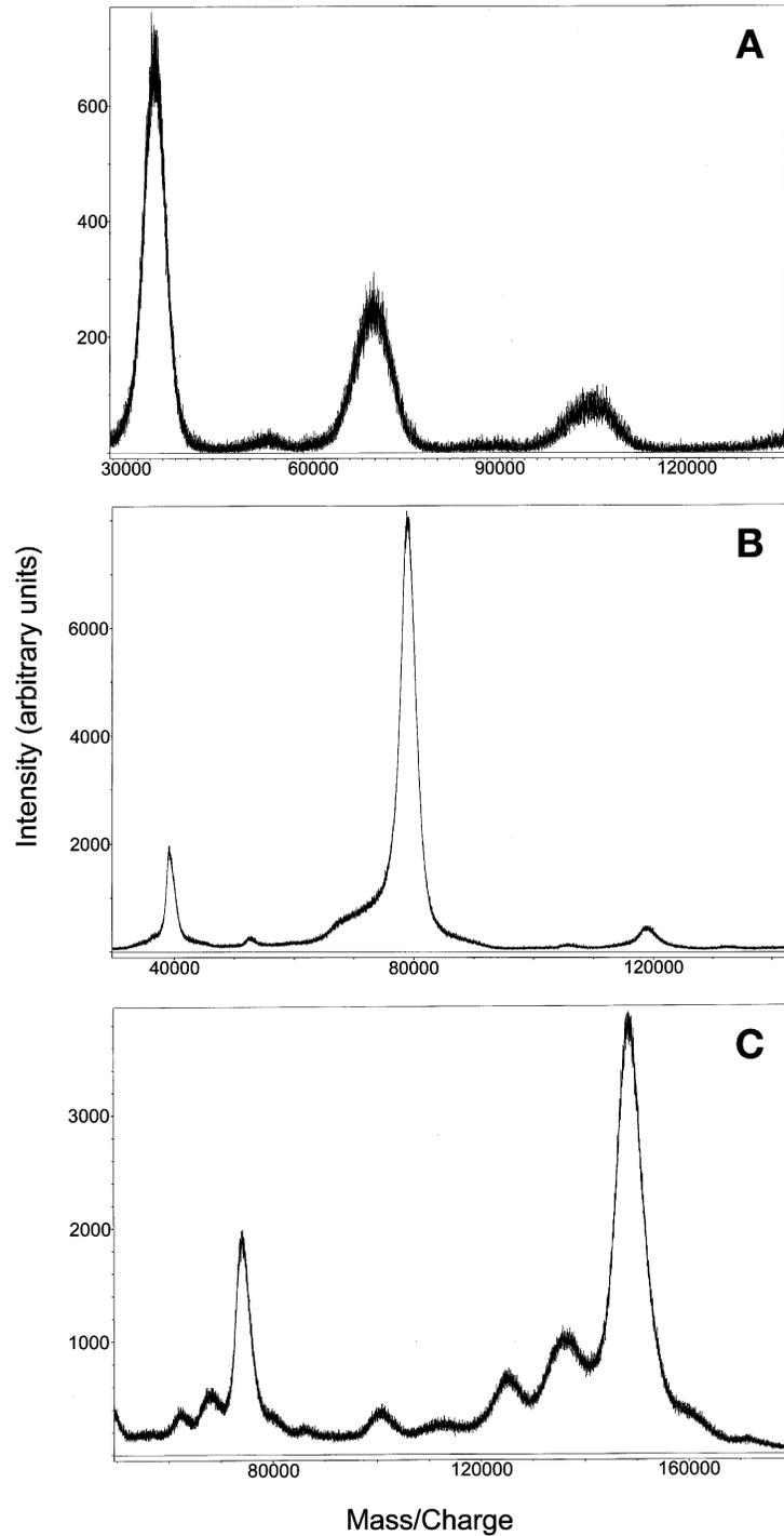
Fig. 1. Matrix-assisted laser desorption/ionization time-of-flight mass spectrometry of  $\alpha_1$ -acid glycoprotein (**A**), transferrin (**B**), and immunoglobulin G (**C**).
