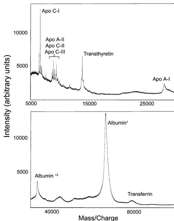
Fig. 3. Matrix-assisted laser desorption/ionization time-of-flight mass spectrometry of diluted serum. **(Top)**  $m/z$  range from 5000 to 30,000 with tentative identification of major peaks. **(Bottom)**  $m/z$  range from 30,000 to 100,000.
